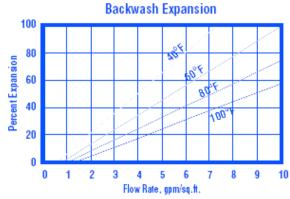
**Backwash:** After each cycle the resin bed should be backwashed at a rate that expands the bed 25 to 50 percent. That will remove any foreign matter and reclassify the bed. The graph above shows the expansion characteristics of Pure PC002 in the sodium form.
